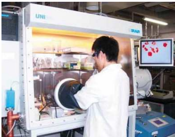
Single Crystal growth of exotic organic functional materials under the oxygen-free condition (< 5 ppm)
