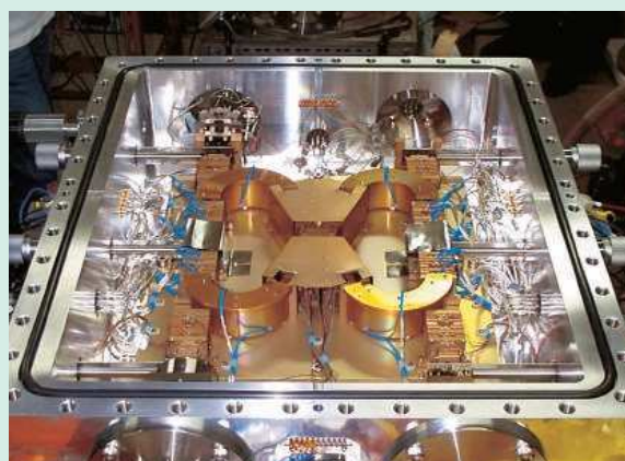
Multi-turn time-of-flight mass spectrometer “MULTUM Linear plus” developed by our group.
