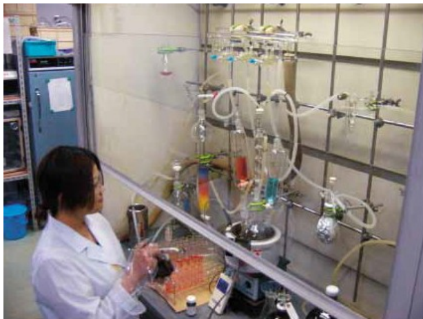
Synthetic organic experiment using exhaust equipment for safety
