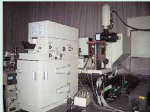
Raman scattering spectrometer with Ar-Kr laser
