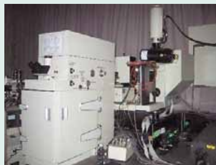
Raman scattering spectrometer with Ar-Kr laser
