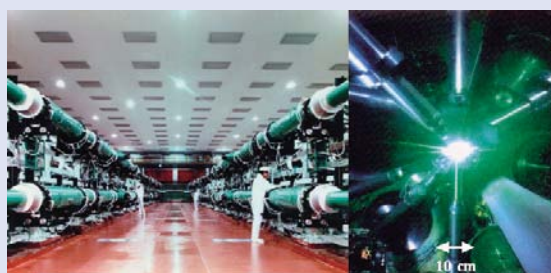
Figures: Left is Gekko-XII laser system and right is the explosion in vacuum chamber in irradiating lasers
